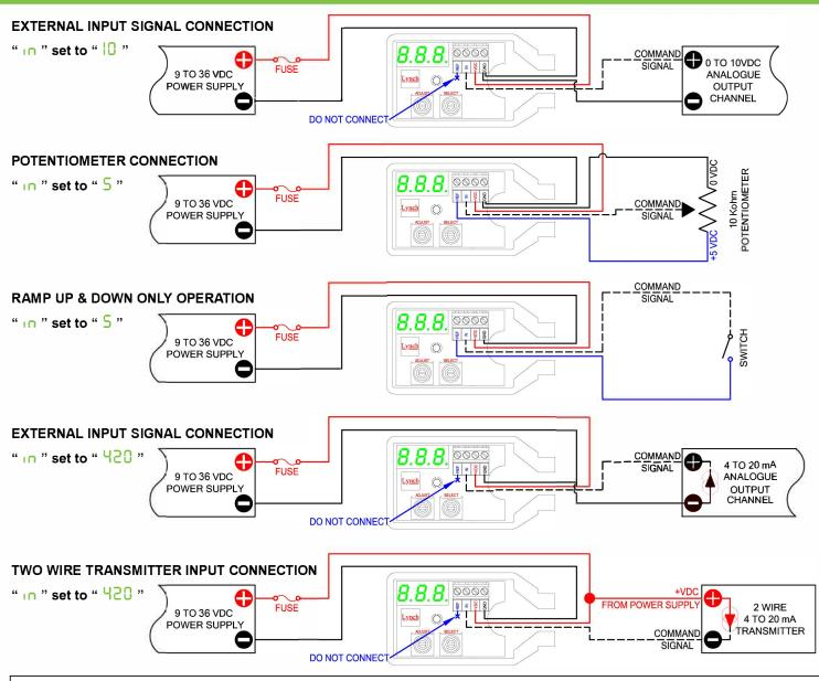
PLEASE NOTE: For "0 to 5 VDC" & "0 to 10 VDC" command input drivers, it is recommended to use independent negative conductors for power supply and analogue output channel (PLC/PC) to maintain command signal accuracy due to voltage drop on long cable runs.
